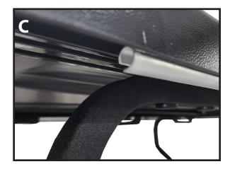
Measure 1  $\frac{1}{2}$ " back from the front of the track, and up  $\frac{1}{2}$ " from the bottom edge of the top and mark for drilling. Using a  $\frac{1}{8}$ " drill bit drill mounting hole and install pop rivet.
