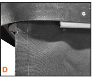
Attach the front valance to the inside face of the aluminum extrusion going across the front of the top using 3 of the self drilling screws. The velcro at the bottom of the valance can be used to attach the valance to the top half of the windshield for better sealing if preferred.
