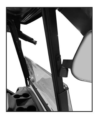
Fold up the windshield and place the upper clips so they are resting against the plastic track. Install a self drilling screw ½" above and ½" below the edges of the clip. Then using the hack saw carefully cut the plastic extrusion to make room for the clip to go between the zippered insert and the strut.
