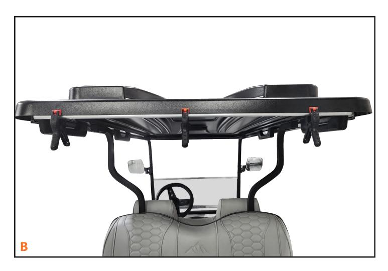
Measure 1  $\frac{1}{2}$ " from each end of the track and  $\frac{1}{2}$ " up from the bottom of the top and drill holes and install pop rivets. Measure 18  $\frac{1}{8}$ " from either end of the track and  $\frac{1}{2}$ " up from the bottom of the top and drill and install the center pop rivet for the rear track.
